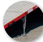
Self-positioning adjustable feet
